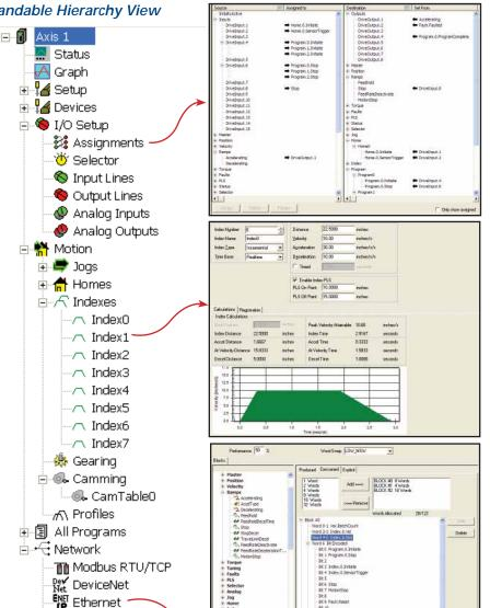
Assignments – Use our "Virtual Wiring" to create programs right out of the box, without writing a single "line of code." For example, on the assignment screen simply drag-and-drop the desired machine function onto the digital inputs and outputs.
